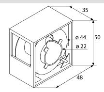
Connector bracket | Socket plate
