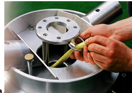
10a. Feed cable through centre and connect to camera allowing min. 180° pan each direction
